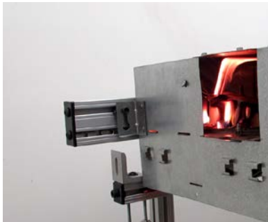
The impeller has ignited and begins to sag onto the motor
