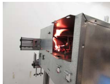
More of the winding wrap and the coating on the winding burns, thus creating a larger flame
