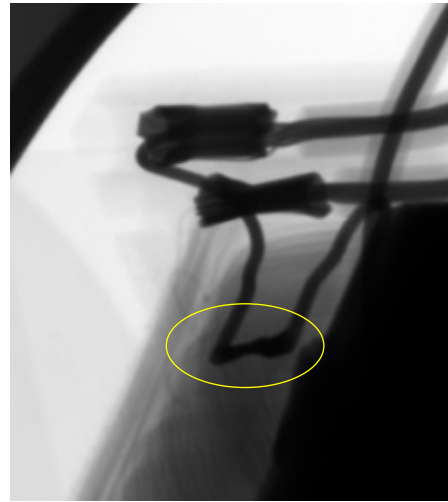
After lock-rotor test
