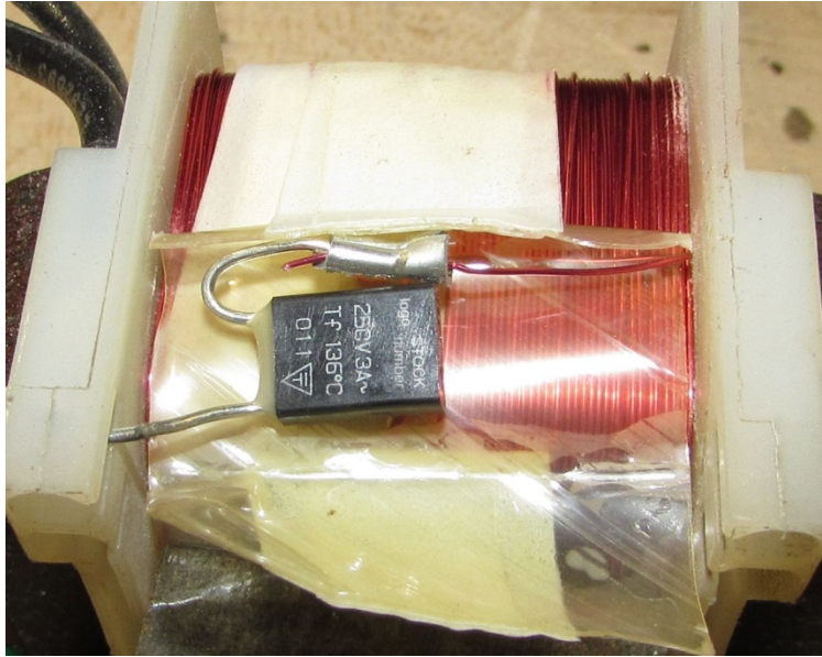
Figure 6. Radial eutectic-type thermal fuse in the sample fans
