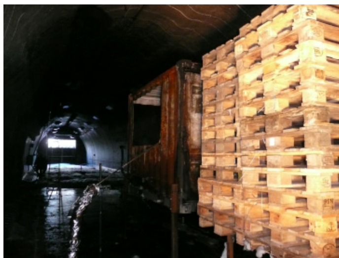
Figure 4 Simulated locomotive and freight wagon loaded with wooden pallets in the If tunnel.
