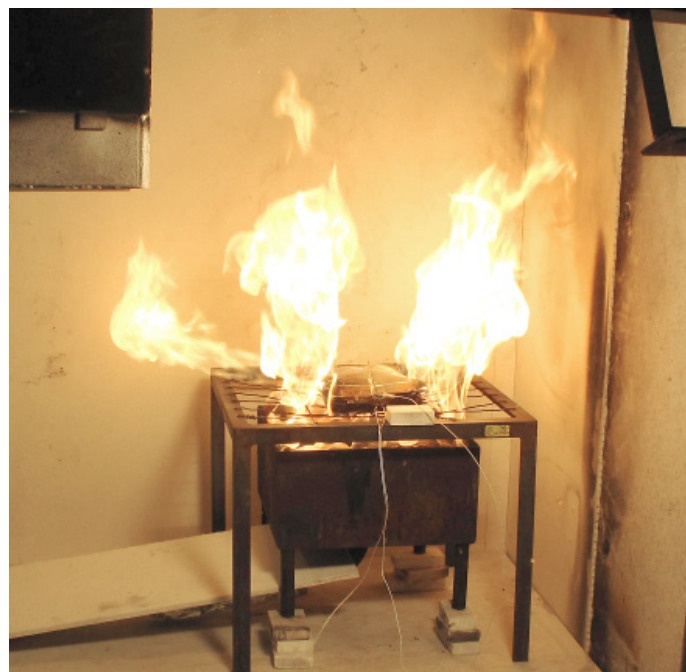
Figure 2 Li-ion 5-cell pack when exposed to a propane flame. Ignited gases from cell venting can clearly be seen.
