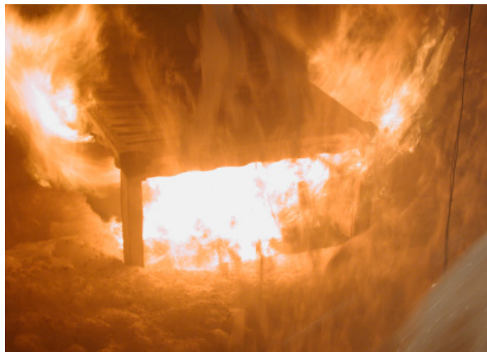
Figure 3 The burning heptane pool when the foam has reached up to the edge of the locomotive's apertures and started to flow in. The fire was extinguished shortly after. At lower application rates, the foam did not manage to get into the locomotive, with the filling rate falling to zero when the foam had reached part-way up the locomotive.
