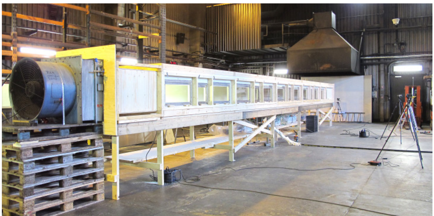
Figure 1 A photo of the 1 m wide model tunnel in scale 1:10.
