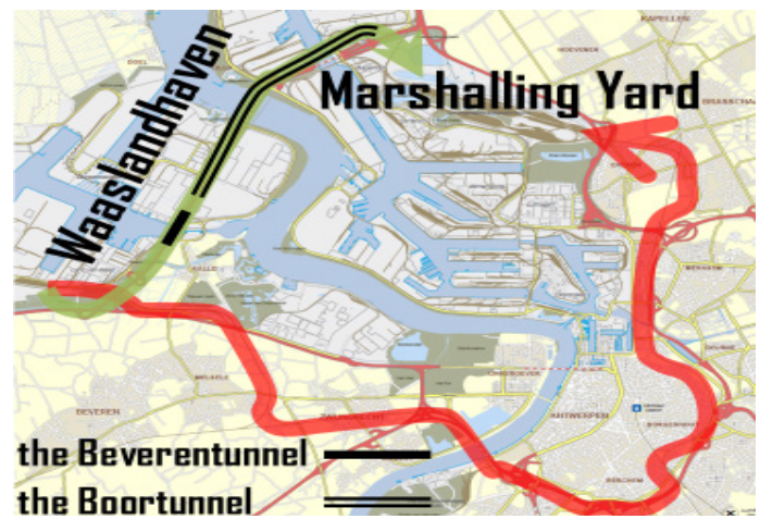
Figure 1 A map of Antwerp's harbour area, showing the new Liefkenshoek Rail Link (green). The black sections show the two tunnels; the twin-track Beveren Tunnel and the double tube Boortunnel. The red route is the earlier connection. Map: By the courtesy of the Port of Antwerp.
