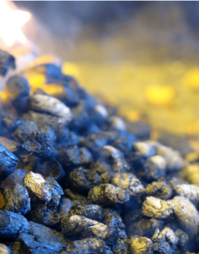
Small-scale fire experiment of wood pellets, performed at the test facility of SP Fire Research AS (Norge).
