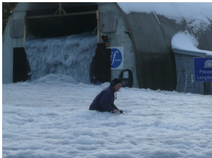
Figure 5 The southern end of the If tunnel after conclusion of a test, showing foam pouring out of the tunnel.
