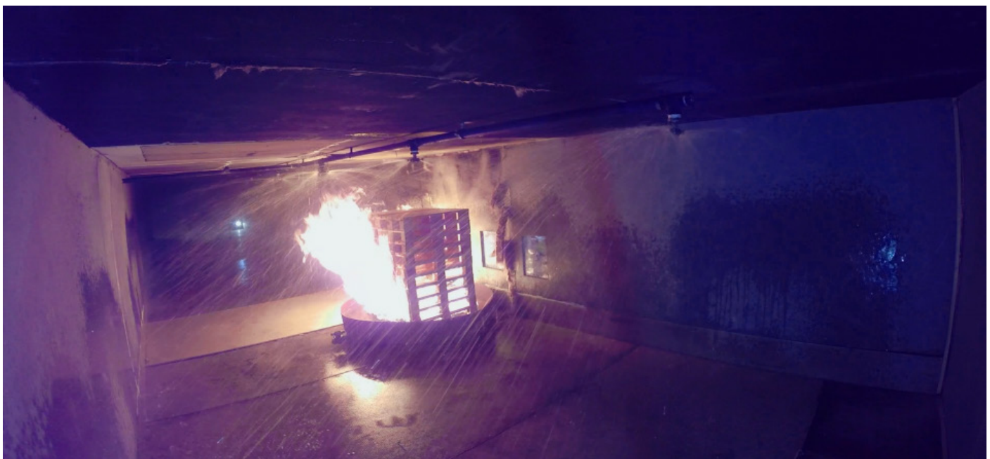
Figure 1 A photo of A wood pallet fire in the tunnel right after activation of the fire suppression system.
