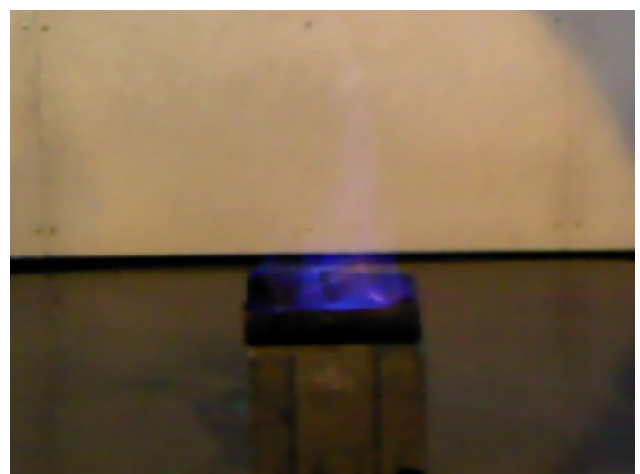
Detection and localization becomes crucial as a methanol fire neither produces visible flames nor smoke.
