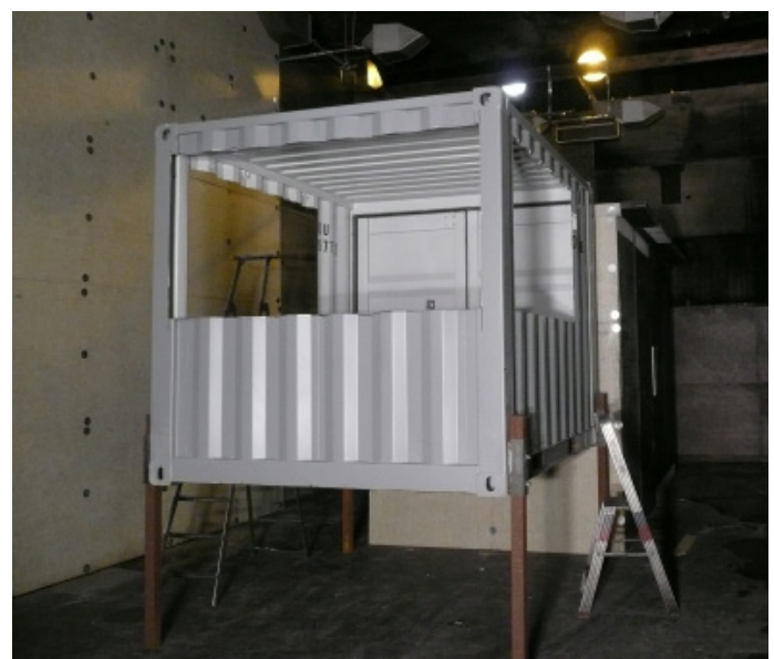
Figure 2 A simulated locomotive and freight wagon in the tunnel section. The 'locomotive' contains a 4,5 m 2 pool of heptane and a diesel oil spray.
