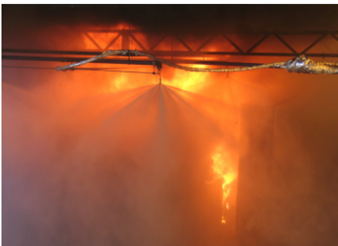
Water mist is not as effective for a fuel with low-flashpoint and wide flammability limits.
