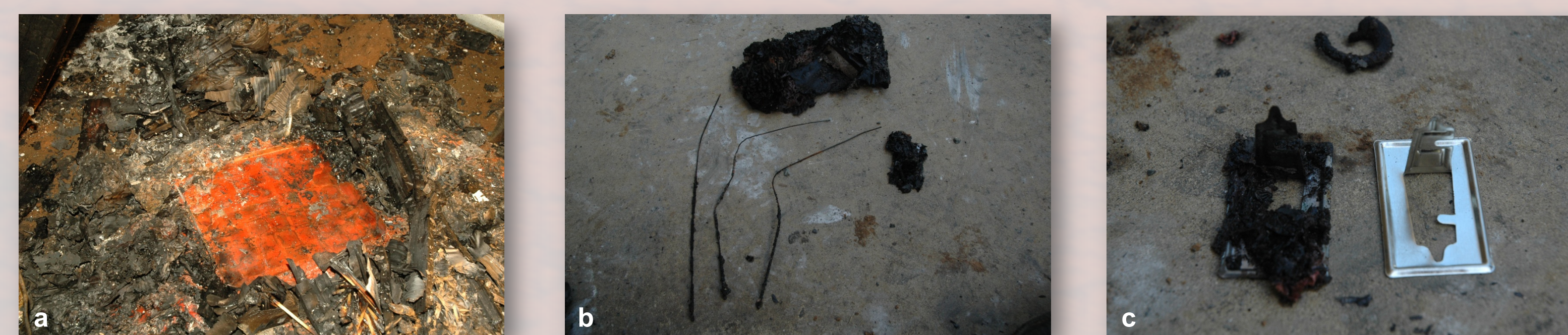
Figure 3: a) during the excavation a crate housing the incendiary device is uncovered, b) sparklers and the remains of matches in molten remains, c) an exemplar mosquito coil holder (from the site) next to the one found in situ.
