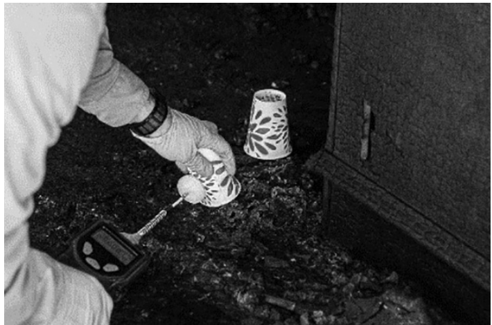
Figure 2. The "headspace cup method" utilizing a paper cup to create a modified head space to increase the concentration of ignitable liquid vapors using the PID. Courtesy of Dan DeMille, Utah Valley University, Provo UT
