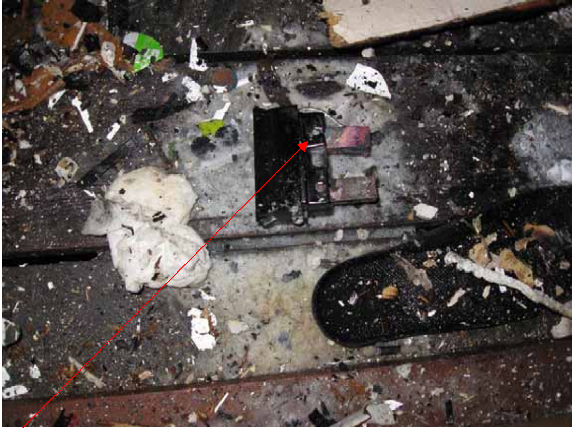
Pin on cut out fuse showing oxidation caused by resistance heating
