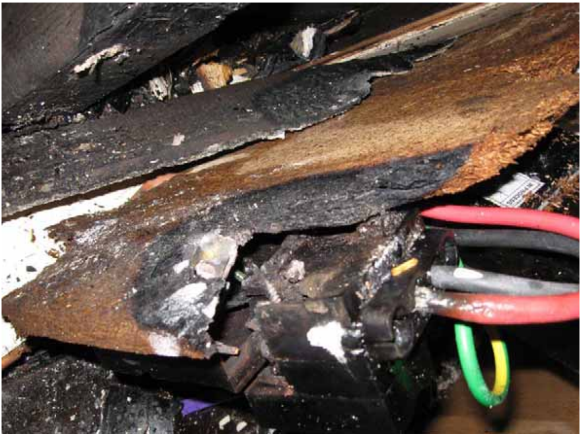
Pin on cut out fuse showing oxidation caused by resistance heating
